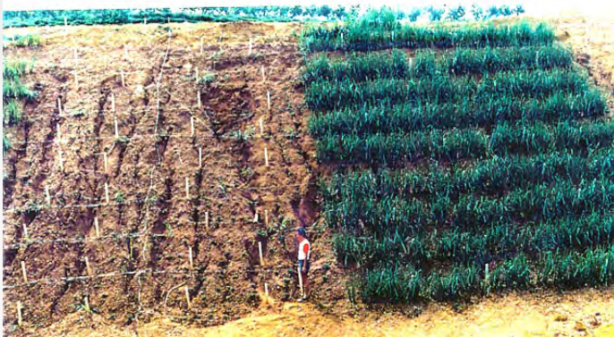
P.K.Yoon's first stabilization trial – vetiver on right, local species on left.
