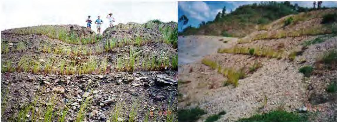
**Figure 52.** Vetiver grew on contours of fresh coal mine overburden.
