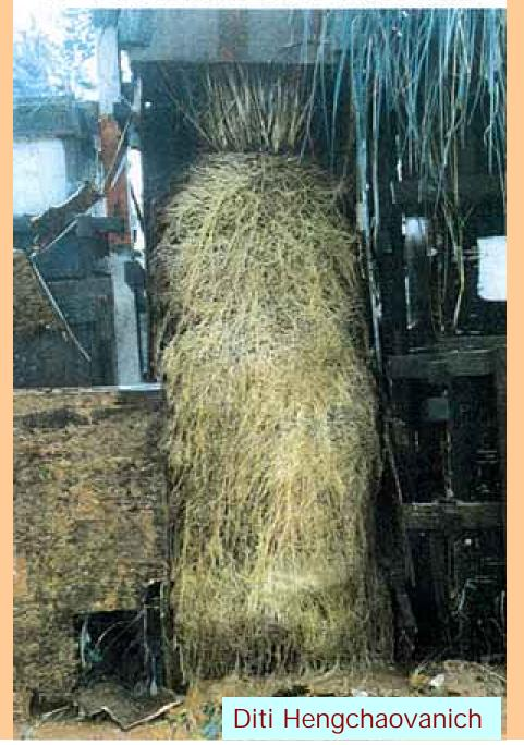
Vetiver roots have the tensile strength of 75 Mpa, equivalent to1/6 strength of mild steel reinforcement.
