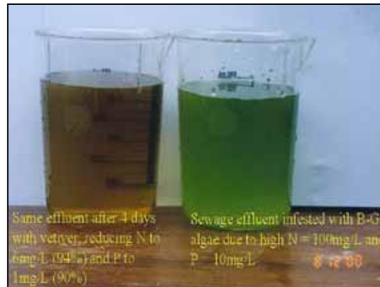
Photo 2: Vetiver cleaned up blue green algae in four days. Sewage effluent containing high Nitrate (100 mg/L) and Phosphate (10 mg/L) (left). Sewage effluent after four days (right). VS reduced N level to 6 mg/L (94%) and P to 1 mg/L (90%).
