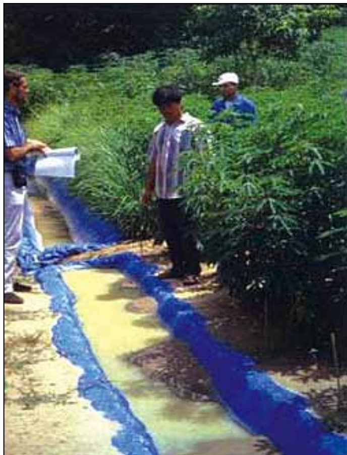
Photo 8: Making soil loss visible (CIAT cassava project). Note difference in rainfall runoff. Less than half in the furthest trap with vetiver protection.
