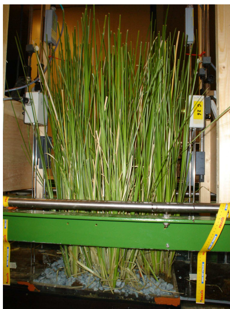
full scale test to simulate run-up through Vetiver
