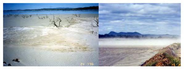
**Figure 43**. A typical large fresh tailings pond of gold mine wastes (left), strong wind causing a dust storm which contains high levels of heavy metals (right).
