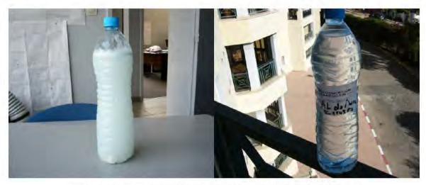
Figure 34. Effluent quality before and after Vetiver treatment.
