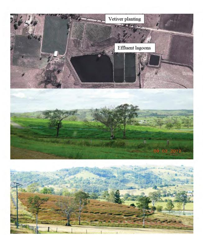
**Figure 24.** Satellite image of Boonah sewage effluent treatment plant assisted with Vetiver grass technology (top), the overview of 4 ha Vetiver planting site at 12 (middle) and 18 (bottom) month old.
