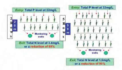
Figure 15. Highly effective in removing Nitrogen and Phosphorus
