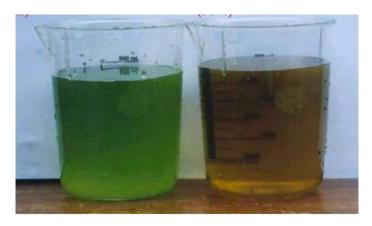
**Figure 9.** High N and P removal capacity of Vetiver: blue green algae infested waste water (left) with high nitrate (100 mg L<sup>-1</sup>) and phosphate (10 mg L<sup>-1</sup>), same effluent after 4 days of treatment with Vetiver (right) reducing N and P level to 6 and 1 mg L<sup>-1</sup>, respectively. Algal infestation was eliminated from the effluent.
