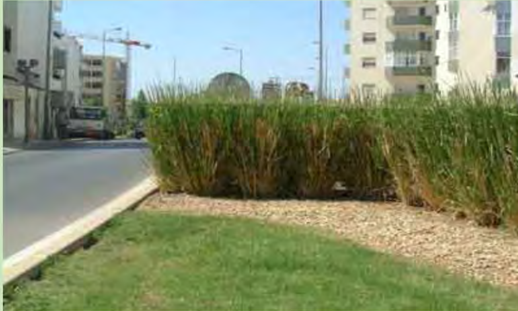
Portugal - Lagos. VS used to prevent head light glare from traffic on a divided road.
