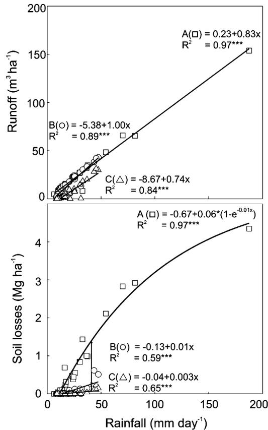
**Fig. 8.** Schematic representations of relationships between runoff and rainfall and between soil loss and rainfall. Lines indicate the situation at establishment of soil conservation measures (A; data from control treatment 2003), the effects of minimum tillage and mulching (B; data from control 2005) and the additional impact of contour hedgerow system (C; average data from hedgerow/barrier treatments 2005).
