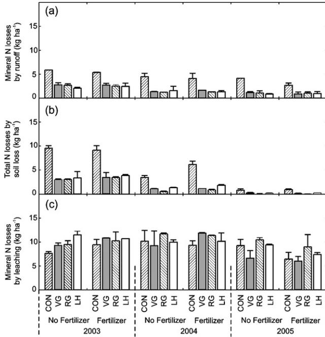
**Fig. 5.** Annual total nitrogen losses by (a) runoff, (b) soil loss and (c) leaching as affected by control (CON), soil conservation measures (VG = vetiver barriers, RG = ruzi grass barriers, LH = leucaena hedge) and fertilizer application during the study period (2003–2005). Error bars denote standard errors.
