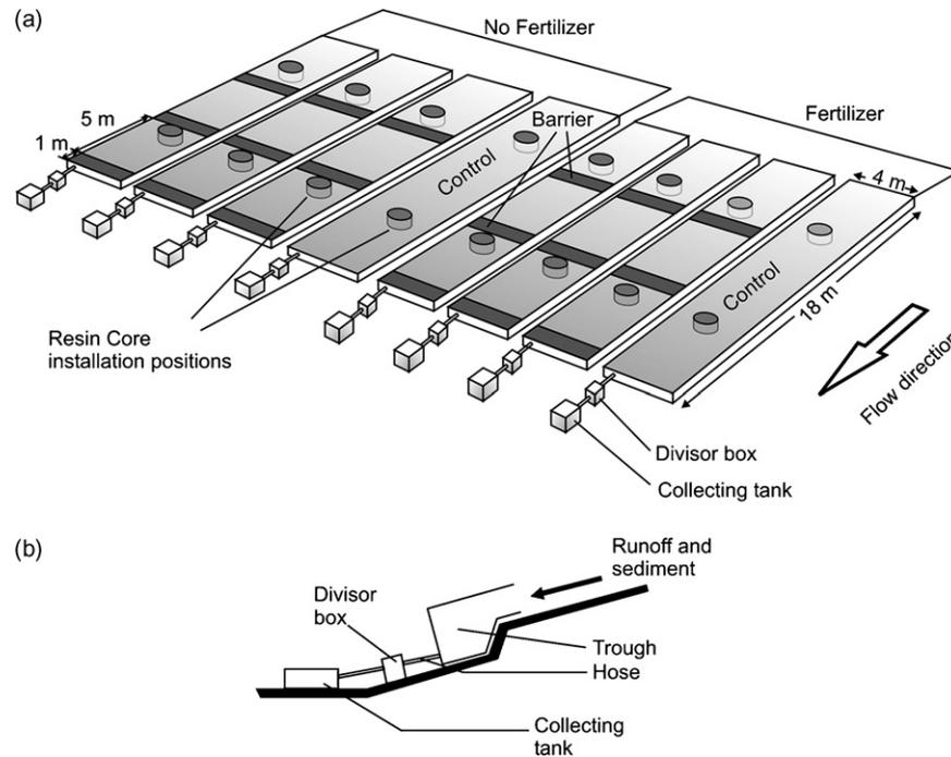
**Fig. 2.** (a) Experimental layout of erosion plots at Ban Bo Muang Noi, Loei province, Northeast Thailand. (b) Schematic of erosion measurement used for collecting runoff and soil loss.
