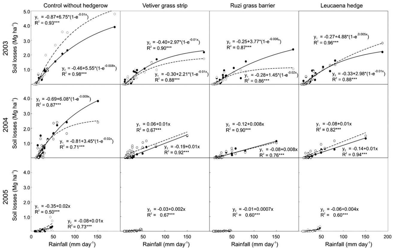
Fig. 7. Relationships between soil loss and rainfall event as affected by soil conservation measure and fertilizer application over the study period (2003–2005). Closed symbols (●) represent datasets from soil conservation measure with fertilizer, whereas open symbols (○) refer to datasets from soil conservation measure without fertilizer. Solid and dashed lines indicate linear fits of results from plots with and without fertilizer, respectively.
