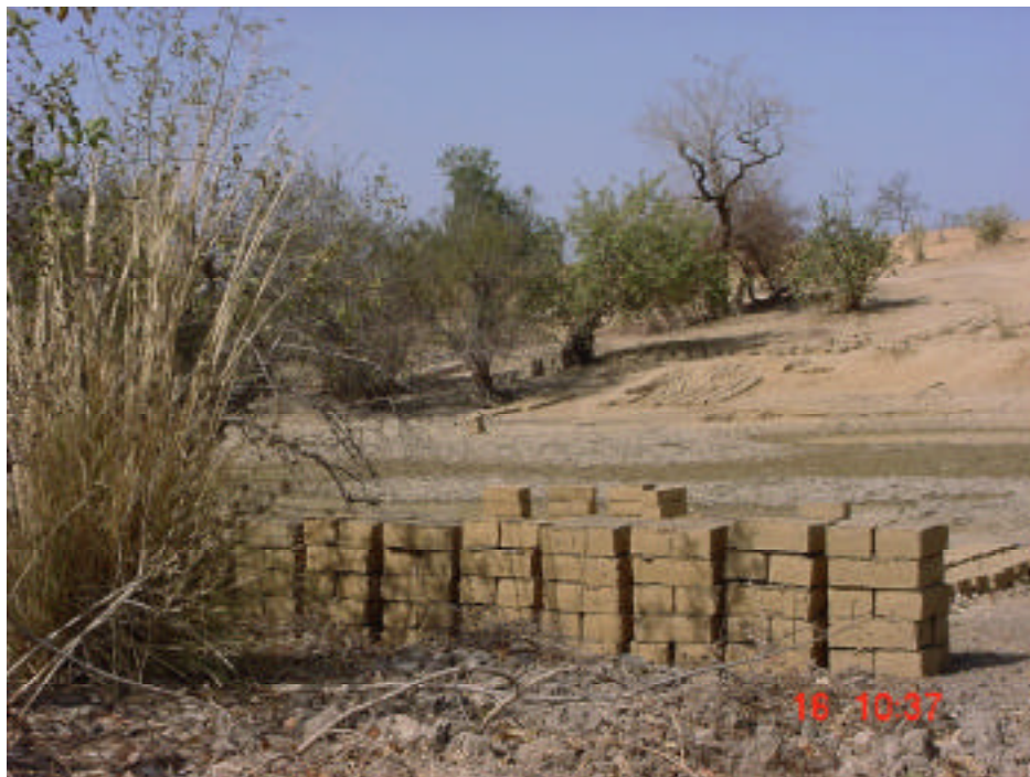
Senegal: v. nigriflora : Baked adobe bricks reinforced with vetiver leaves (clump on left). Users claim vetiver reduces fissures and cracking in constructed walls.
