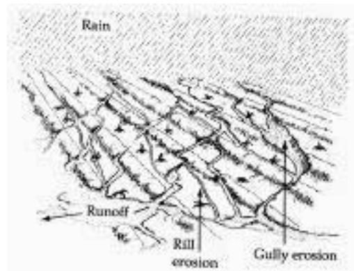
Figures 7-15a and 7-15b illustrate what happens when the two farming systems are exposed to heavy rainfall. Farmer A's field is protected by the vegetative hedges, and there is no loss of soil (Figure 7-15a). The contour furrows store all the rainwater they can hold. Any surplus rainfall runs off, but the vetiver hedges control the flow—slowing it down, spreading the water about—and cause the silt to be deposited. As a result, the runoff is conducted down the slope in a safe, nonerosive manner.
