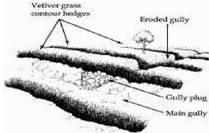
The same would apply to normal gullies as shown in Figure 7-34a. Once established, the grass would fill and terrace the gullies with silt. In an upland area of Fiji, as shown in Figure 7-34b, a gully was stabilized with vetiver grass some 30 years before the photo was taken. In the photo, the gully is fully stable and the hedges remain where they were originally planted.
