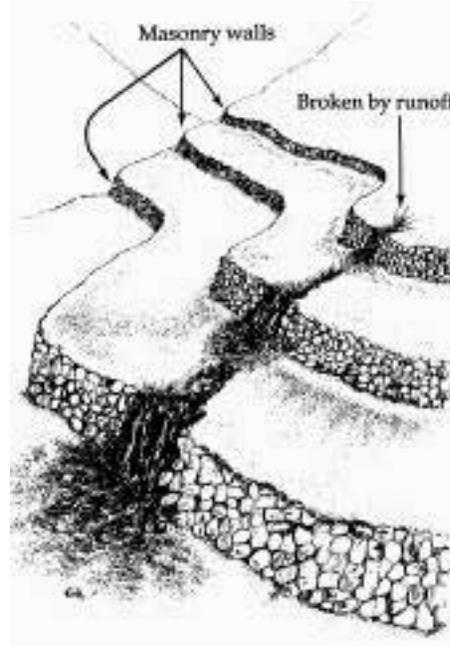
**Figure 7-31c.** Vetiver grass, planted on the extreme edge of each terrace, stabilizes the terraces without interfering with the essential drainage between the stones.
