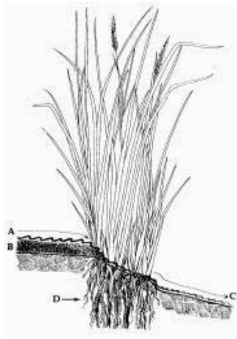
**Figure 7-11b. This cross-sectional view of a two-year-old vetiver hedge shows how about 60 cm of soil has been trapped above the original dark band of topsoil.**
