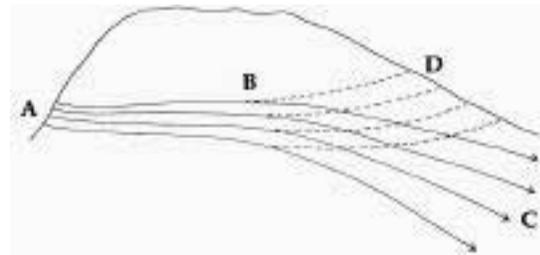
**Figure 7-13c. Earth banks, which must convey the runoff to a waterway off to the side of they field, must be constructed on the exact contour (marked with pegs at A), often making it difficult for the farmer to follow when plowing. With vegetative hedges, however, the contour can be averaged into a smooth curve (line B).**
