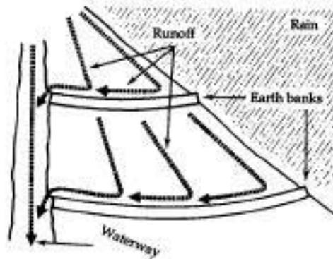
Figure 7-7 shows the unnatural way the land is drained by the constructed system. All of the runoff is channeled sideways and dumped into a constructed but unproductive waterway that no smallholder would want running through his or her farm. This system makes the areas below the banks too dry and the channel areas too wet for optimum crop production.
