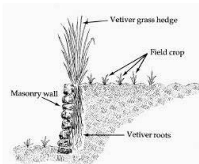
**Figure 16-5a.** This vetiver hedge is ideal for crop production. The farmer, using the hedge as a guideline, plowed on the contour. The combination of the hedge and plowing on the contour will give maximum moisture conservation, while preventing erosion.
