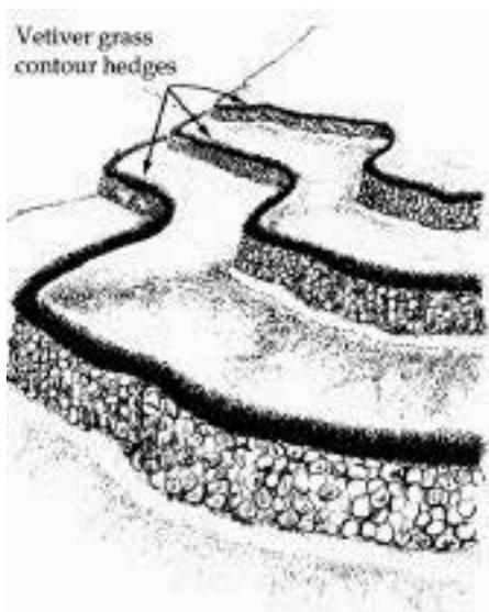
**Figure 7-31d.** The vetiver root system stabilizes the entire rock face of the vulnerable masonry risers.
