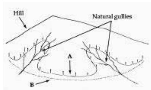
A true contour embraces all slopes, major or minor; it is a line of equal elevation around a hill. The furrows in Figure 7-13a, which starting from point A, follow the main slope straight down to point C, instead of curving around the hill; they are not on the contour and therefore will neither
