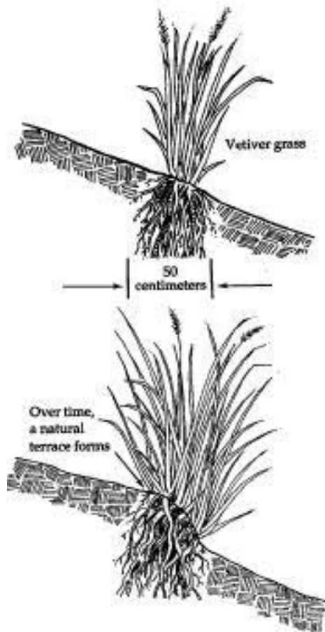
**Figure 7-8b.** Soil build up naturally behind this vetiver hedgerow. This photo is a cross section of a hedge and soil profile. Note the original soil surface is shown as the dark humic layer.
