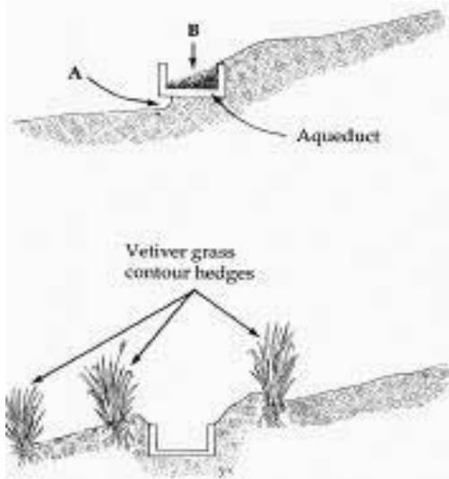
**Figure 7-37b.** On a sugar farm in Zimbabwe, a vetiver hedgerow protects an irrigation channel (behind the hedge), while other rows protect the drain.
