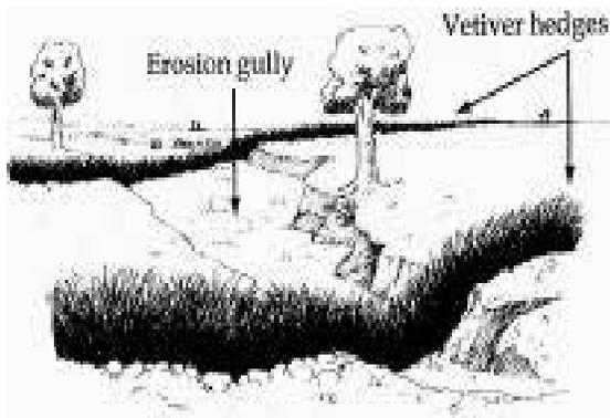
**Figure 7-34b. In this upland area of Fiji, some 30 years before this photo was taken, this gully was stabilized with vetiver hedgerows, which still remain where they were originally planted.**
