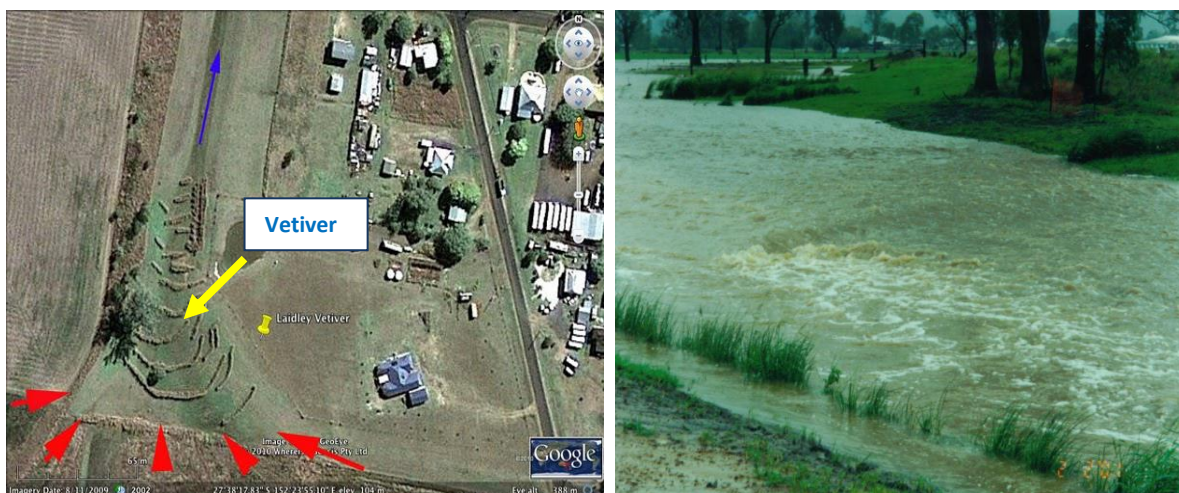
Layout of vetiver rows at the head of the drain and flood flow at 5m/sec
