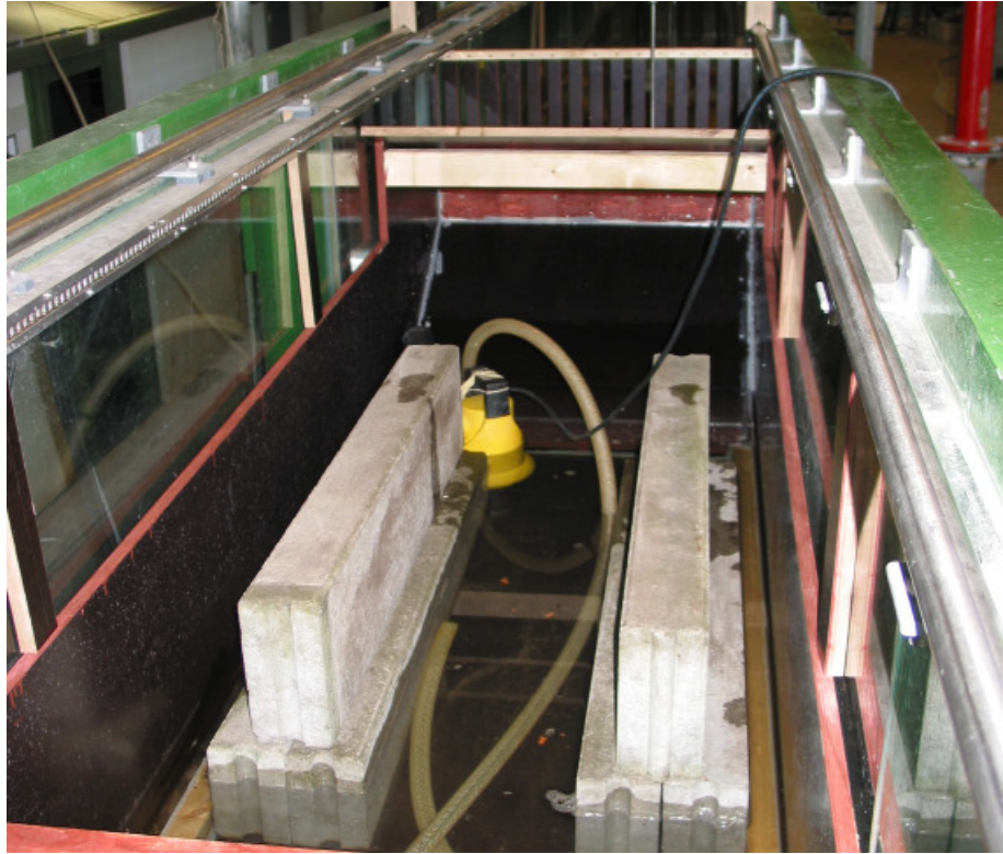
Figure 3.6 The box that was used to collect the water. The pump was used to pump water to a weighing device. In the background the hedge is visible.
