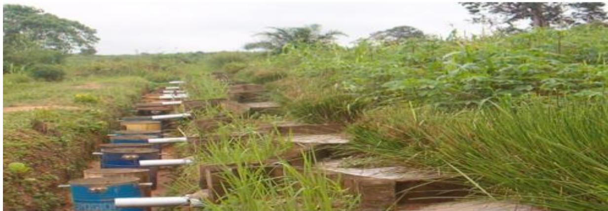
Figure: Experimental setup with vetiver buffer serving as an erosion control measure in Cross River state-Nigeria (Oku et al. , 2015)
