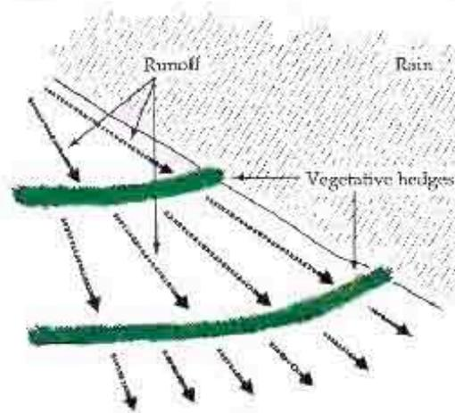
**Reducing flow velocity, spreading runoff water, trapping sediment**
