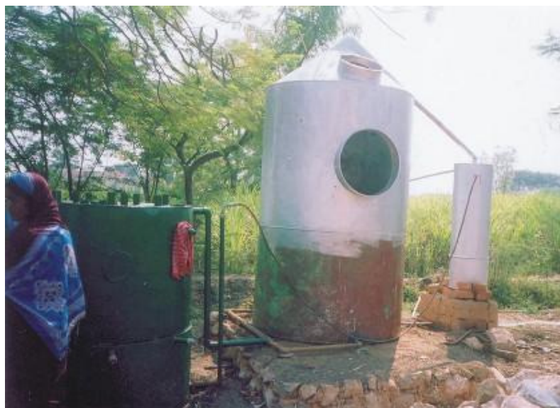
Plate 4: Small scale vetiver processing unit
