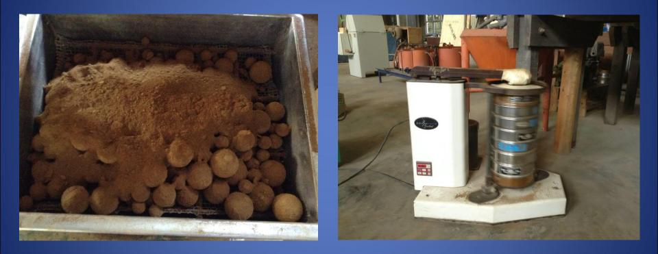
Figure 4. Particle size reduction by Ball Milling, and RoTap and sieving.
