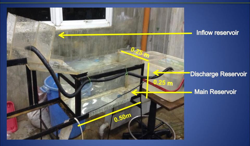
Figure 5. Experimental Set-up without Vetiver System, without silt. Baay. Tan., Philippines. 2015
