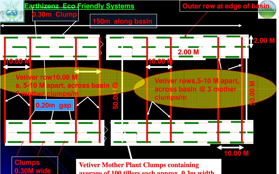
vetiver Mother Plant Clumps containing average of 100 tillers each approx. 0.3m width with 0.20 clear gap between clumps. Distance between rows= 2m
