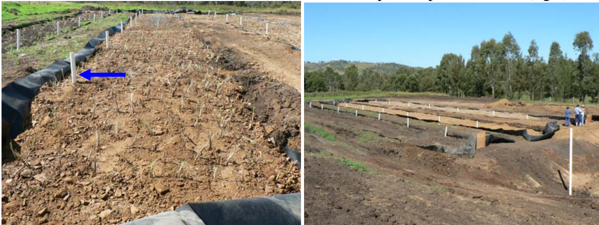
Photo 3: SBRB with Piezometers (left) and the complete experimental site (right)
