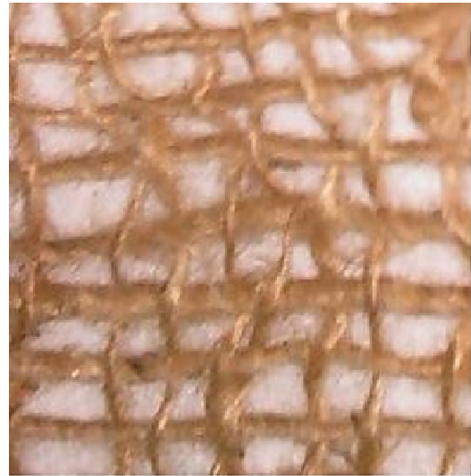
Fig. 5 Photograph of geo-jute used in the field trail of slope protection
