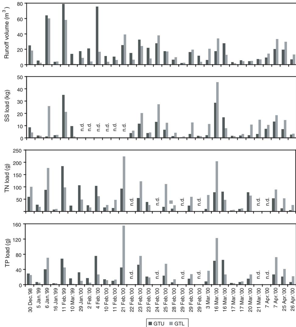
**Fig. 6.** Runoff volumes and suspended material loads at Gallagher's Tree Upper (GTU) and Lower (GTL) flumes for each of the paired events (summarised in Table 3, 4); n.d., no data.
