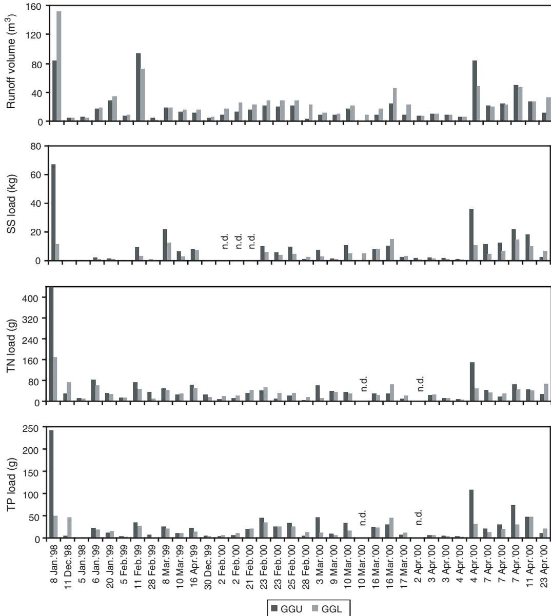
**Fig. 2.** Runoff volumes and suspended material loads at Gallagher's Grass Upper (GGU) and Lower (GGL) flumes for each of the paired events (summarised in Tables 3, 4); n.d., no data.
