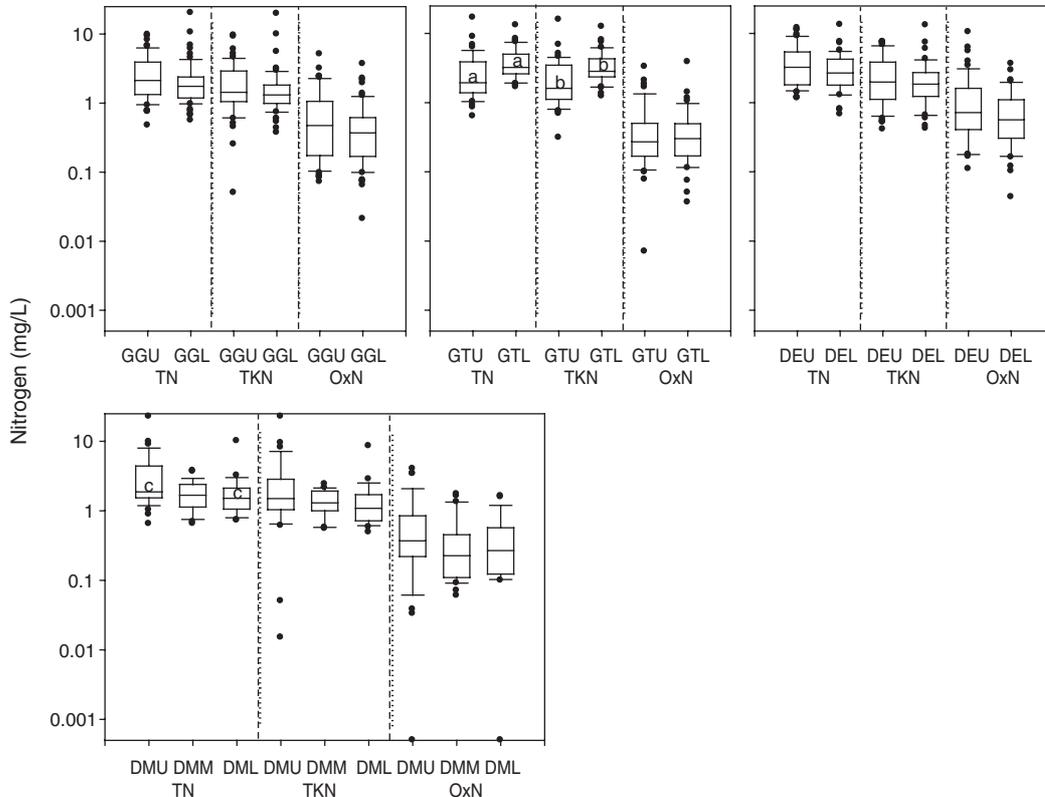
**Fig. 4.** Nitrogen concentrations for all composite and individual samples analysed for the Upper (U) and Lower (L) sites at Gallagher's Grass (GG), Gallagher's Tree (GT), Dunne's Extreme (DE), and Dunne's Moderate (DM). Medians with the same letter are significantly different ( $P < 0.05$ ).
