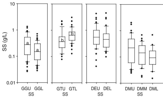
**Fig. 3.** Suspended sediment concentrations for all composite, flow weighted mean concentration and individual samples analysed for the Upper (U) and Lower (L) sites at Gallagher's Grass (GG), Gallagher's Tree (GT), Dunne's Extreme (DE), and Dunne's Moderate (DM). Note only one sample per event. Box represents the median with 25th and 75th percentiles, whiskers are the 10th and 90th percentiles and outliers are dots. Medians with the same letter are significantly different ( $P < 0.05$ ).
