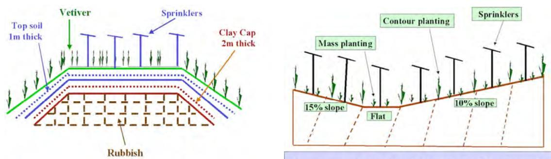
**Figure 1: Cross section (left) and longitudinal section (right) of the Stotts Creek landfill mound**
