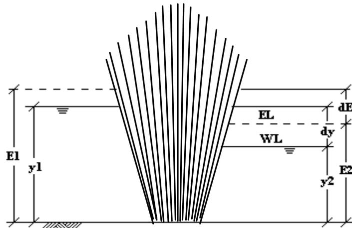
**Figure 1:** System of flow through a vetiver grass hedge and definition of terms in the discharge-depth equation
