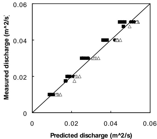
**Figure 3:** Predicted vs measured discharges for the July 1994 trial,  $r^2 = 0.963$  ( $\Delta$  Hedge 1;  $\bullet$  Hedge 2;  $\blacksquare$  Hedge 3)
