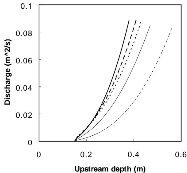
**Figure 4:** Plots of Equation 2 for each of the trials for a downstream depth  $y_2$  of 0.15 m (— March '93; - - July '93; ··· Sept '93; - · - Dec '93; - - - July '94). The hedges tested in July 1994 (which were then 20 months old) appeared to have sufficient retardance at least for effective use on the flood plains. The authors have no indication of
