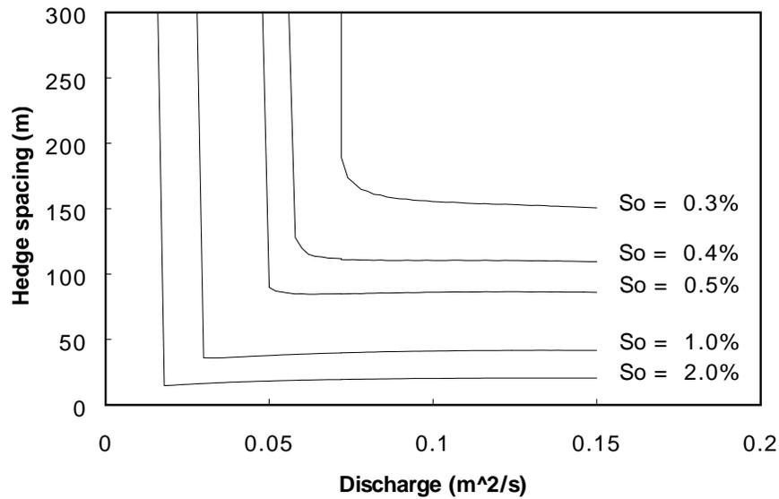
**Figure 6:** Effect of land surface slope,  $S_o$  on hedge spacing for a  $V_{max}$  of 0.5 m/s and Manning  $n$  of 0.03
