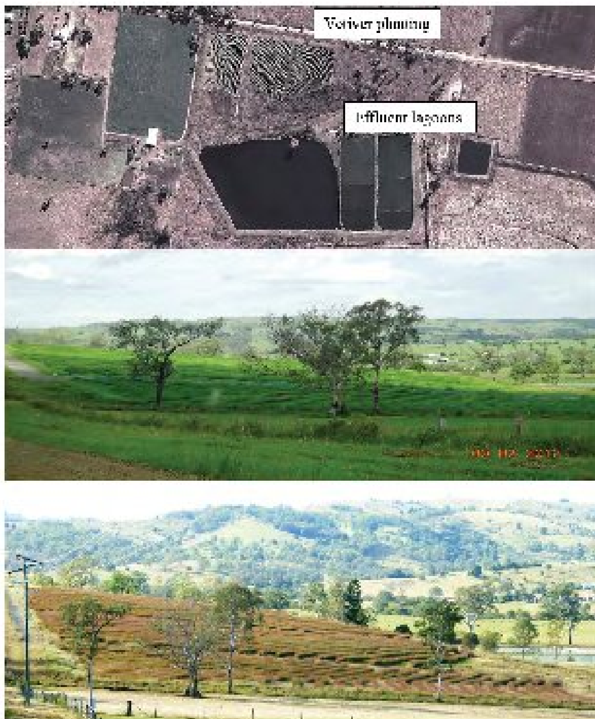
Figure 24. Satellite maps of Iteash sewage effluent treatment plant assisted with Veriver grass technology (top), the overview of 4 ha Veriver planting site at 12 (middle) and 18 (bottom) month old.
