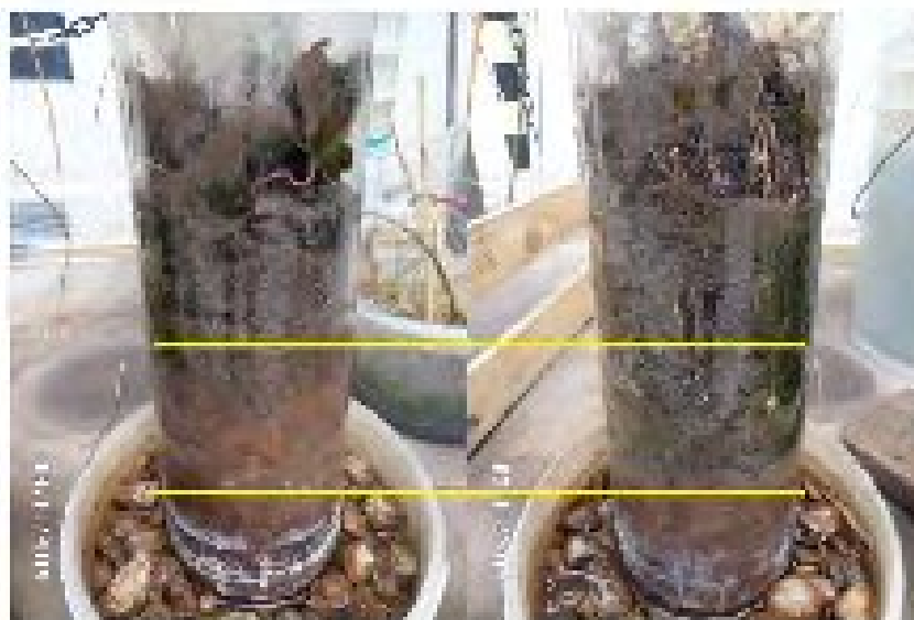
Figure 7. The colour of the soil layer changed when the roots penetrated into the contaminated soil.
