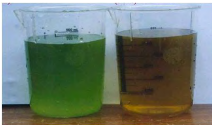
Figure 9. High N and P removal capacity of Vetiver: blue green algae infested waste water (left) with high nitrate (100 mg L -1 ) and phosphate (10 mg L -1 ), same effluent after 4 days of treatment with Vetiver (right) reducing N and P level to 6 and 1 mg L -1 , respectively. Algal infestation was eliminated from the effluent.
