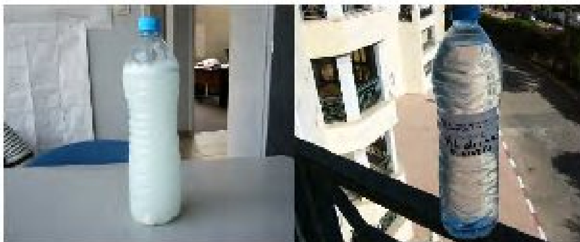
Figure 34 Effluent quality before and after Vetiver treatment
