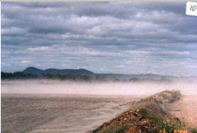
Australia: New gold mine tailings showing wind blown dusts laden with arsenic and other heavy minerals. Photo Credit -- Paul Truong
