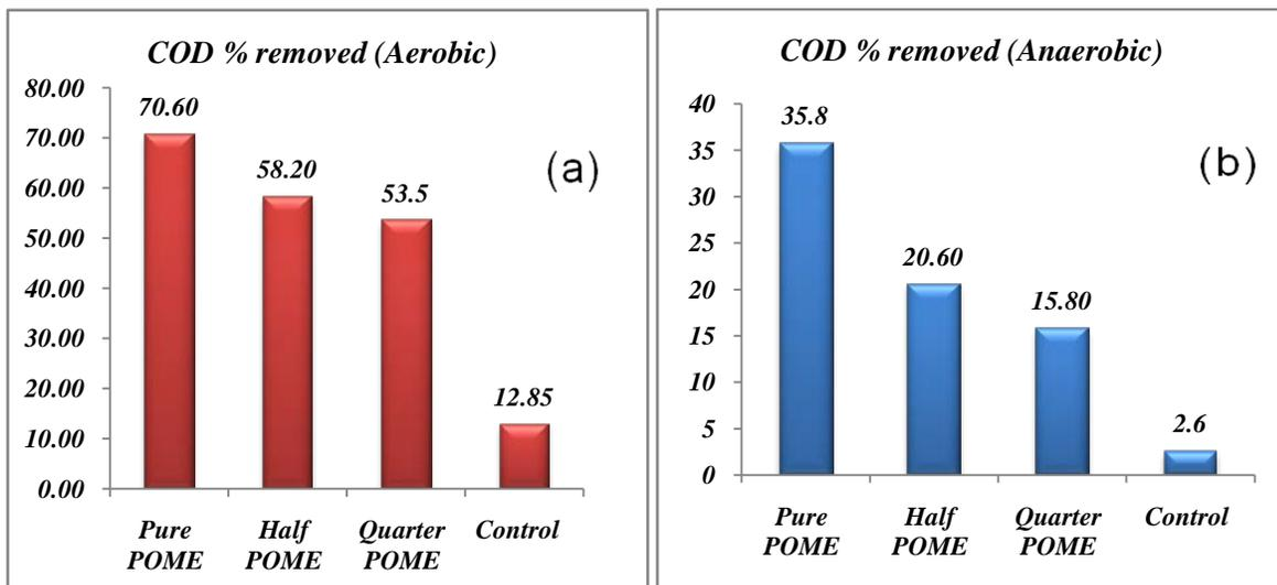
**Figure 2: (a) Reduction of COD in Aerobic set up (b) Reduction of COD in Anaerobic condition.**
