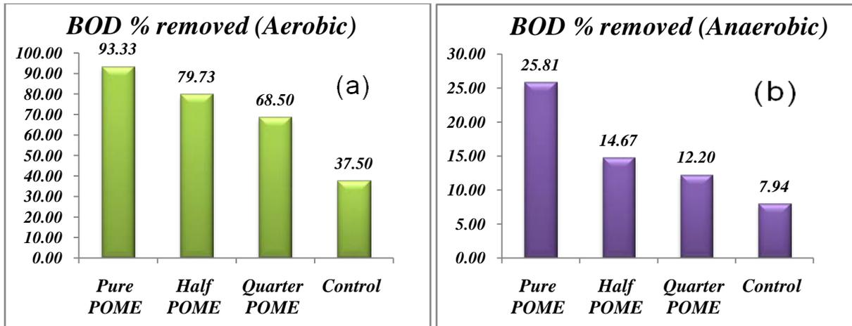
**Figure 1: (a) Reduction of BOD in Aerobic set up (b) Reduction of BOD in Anaerobic condition.**
