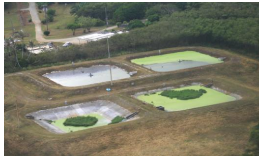
Fig.1: Aerial view of Inarajan sewage treatment plant before planting the Vetiver grass in May 2008. The general process description of the Inarajan treatment plant, including liquid and solid streams, is as follows (GWA, 2006):
