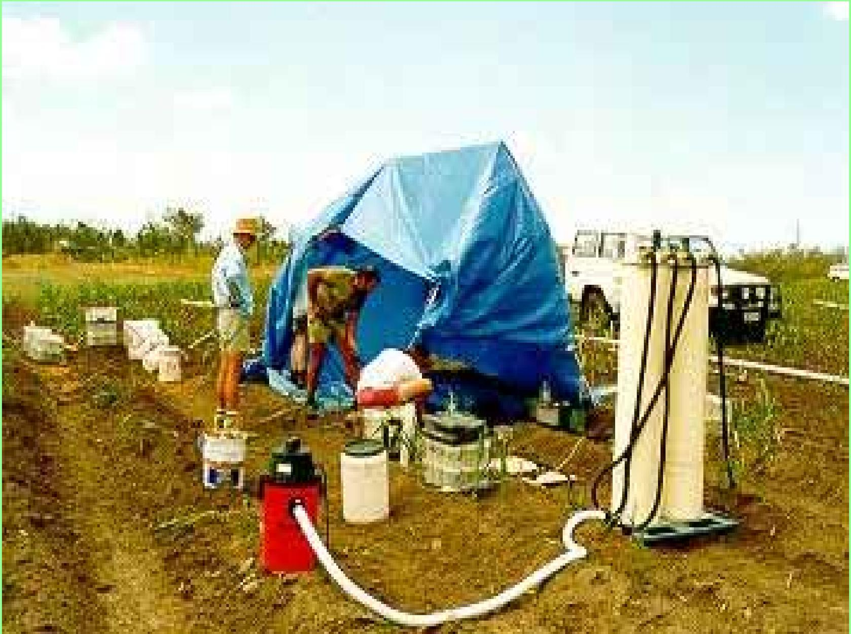
Trial being set up to determine the efficiency of vetiver hedges in trapping nutrients and agrochemicals in a sugarcane field
