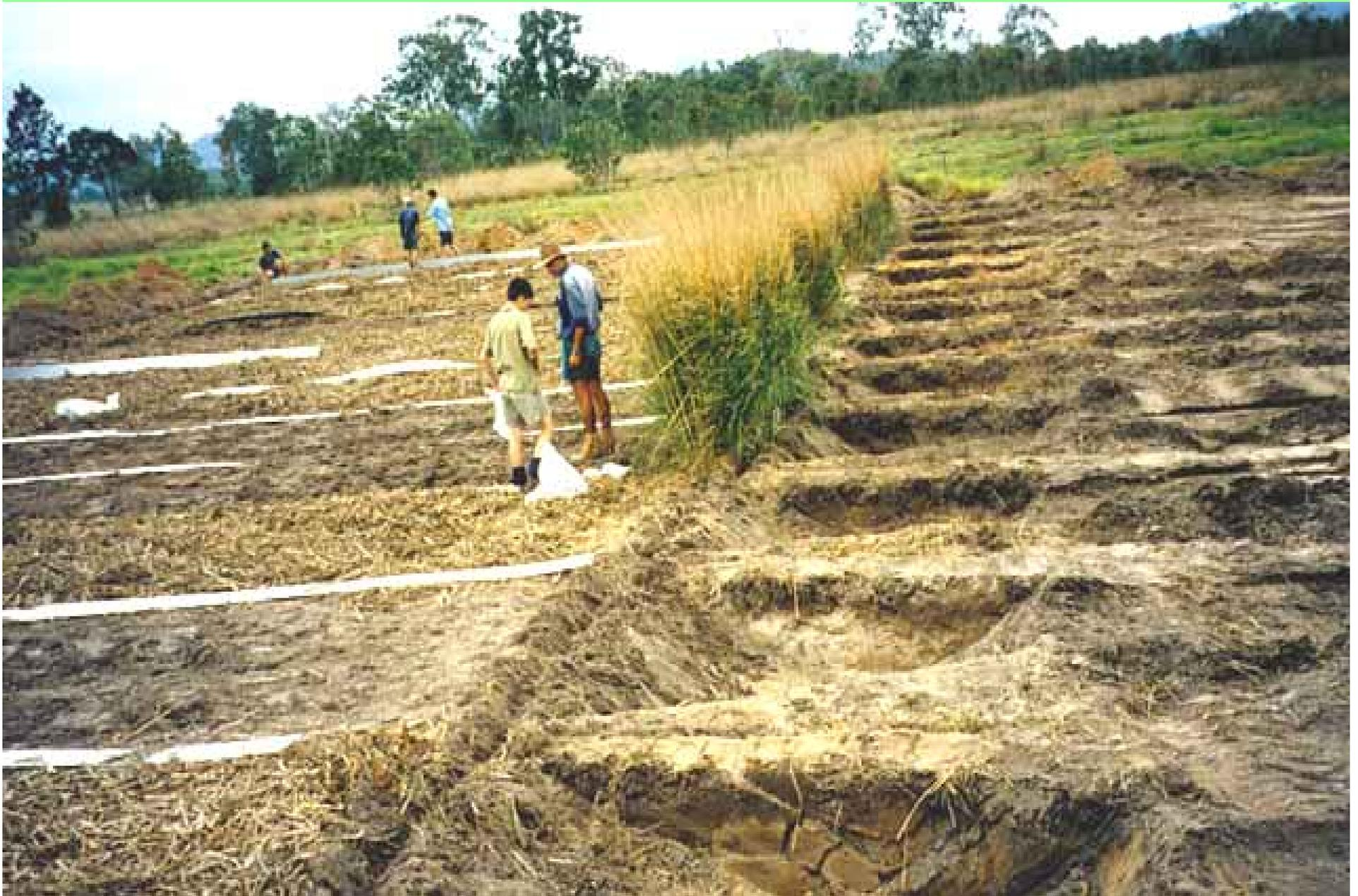
Trial being set up to determine the efficiency of vetiver hedges in trapping nutrients and agrochemicals under different management systems
